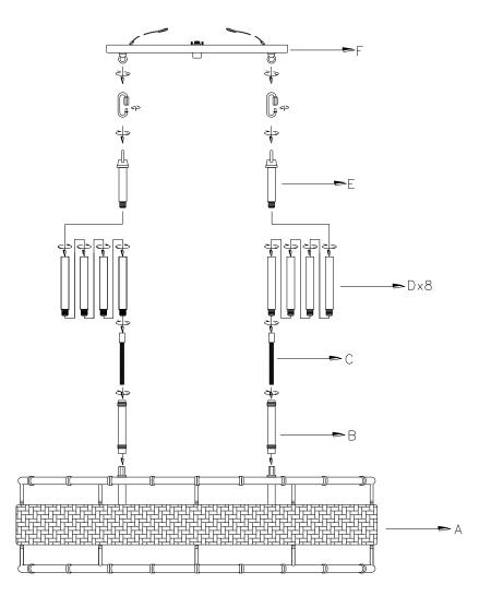
$B \to A \to C \to D \to E \to BULB$
