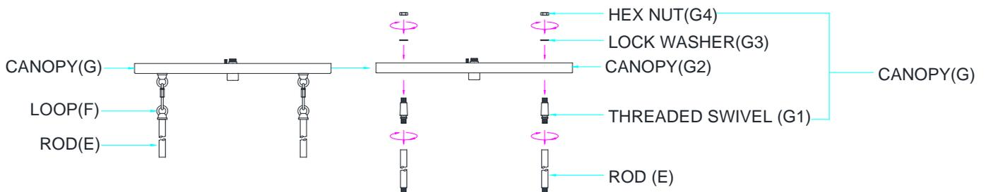
1. Remove the loop, lock washer, and hex nut from the canopy (G). Remove rod (E).
