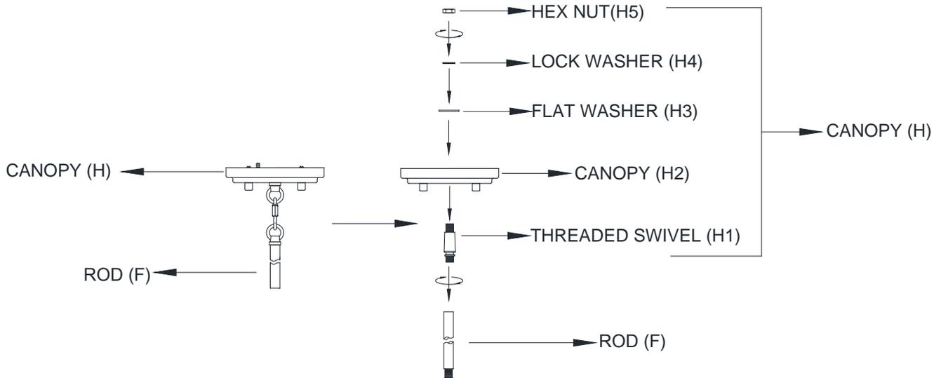
1. Remove the loop, flat washer, lock washer, and hex nut from the canopy (H) and rod (F).
