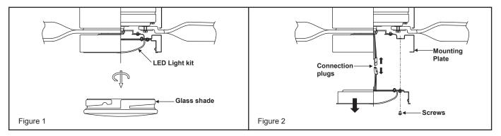
3. While holding the new LED light kit under your fan, make the polarized plug connections. (Fig. 3) - Red to white - Black to black
