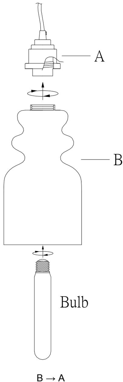
1. Carefully unpack and identify all parts referring to illustration for parts identification.
